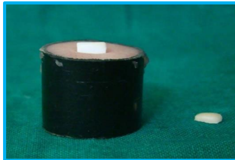
Fig. 3: Sample after subjecting to shear load in universal testing machine
