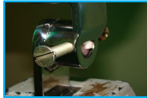
Fig. 2: Sample mounted in jig, subjected to force by universal testing machine
