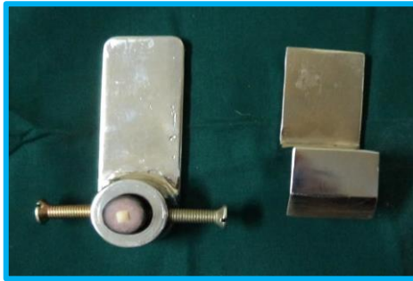
Fig. 1: A customized jig with sample placed in PVC pipe using cold cure acrylic
